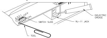
Coat reader connector with the silicone grease supplied to seal off moisture for outdoor mounting. To avoid having ESD (electrostatic discharge) interfering with the operation of the reader, the reader casing shall be grounded. This can be accomplished be tying the mounting bracket to earth ground locally (e.g. grounded conduit).
